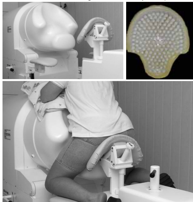
Figure 1. SARA, consisting of 151 gradiometers arranged to comfortably fit the gravid abdomen.
