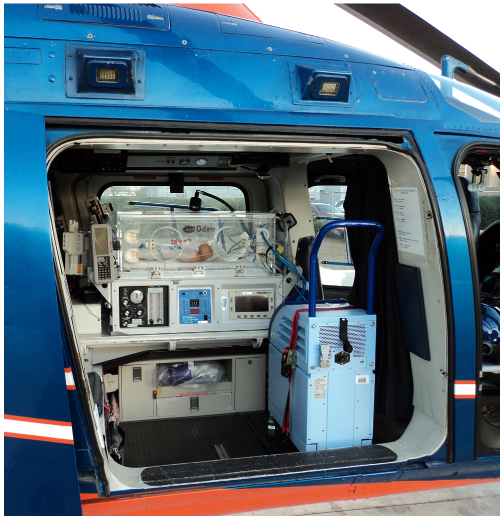
Figure 3. The configuration for transport in helicopter at Shands-UF is shown. The CritiCool™ unit is placed behind the pilot's seat and secured.
