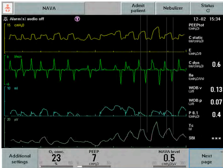
Figure 3. This shows that the ventilator adjusts the level of support proportional to the infant's inspiratory effort during invasive ventilation in the NAVA mode. Compare the last four tracings on the right in the bottom "green" tracing to the similar ones on the top "yellow" tracing.
