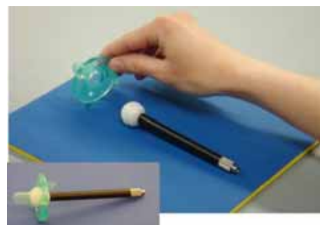
Figure 2. Soothie and pacifier receiver with Luer cannula for intraluminal pressure transduction.
